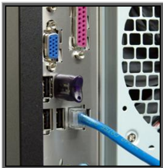
Image 1-2: An audible "click" is heard when the Network Cable is inserted correctly
