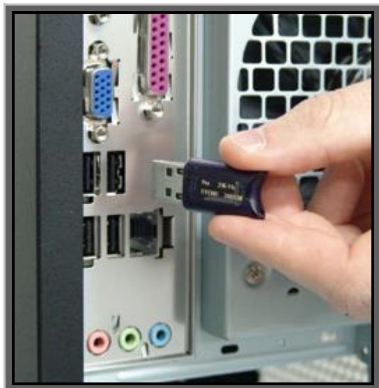
Image 1-1: Inserting a USB license key into a spare slot
