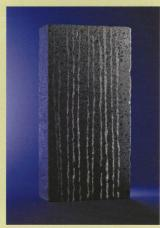
This dense, impact-absorbing silicone has important safety applications. It's only an inch thick, but you can drop an egg on it and the egg won't break. It could be used to make car
